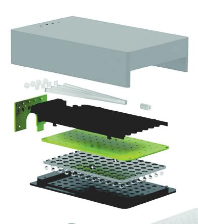
The Absorbance 96 is the first microplate reader on the market to contain 96 individual detection units. This means that all wells can be read simultaneously — in parallel — allowing for extremely fast photometric measurements. Without the need to scan across multiple wells, the Absorbance 96 has no moving parts. In combination with long-life LEDs, this solid-state design provides a maintenance- free user experience and ensures reliable, high quality results.
