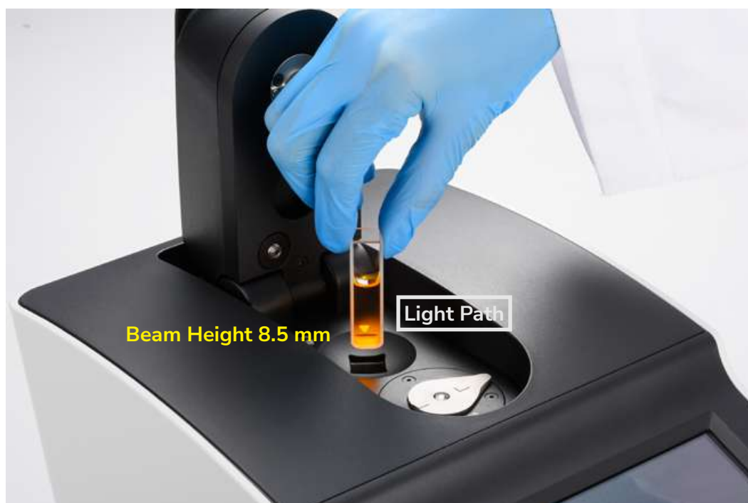
Figure 11. The Light Path Arrow and Beam Height of Cuvette Holder (1000C only)
