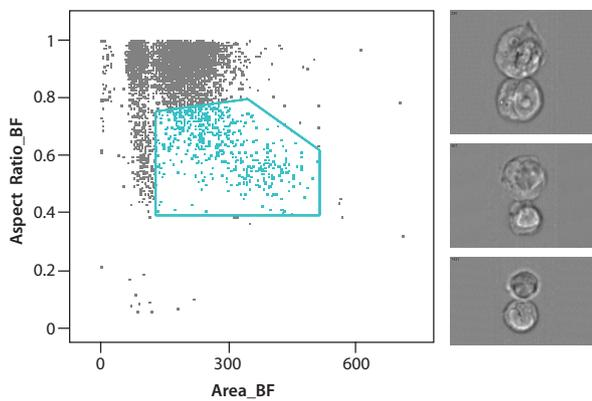
**Step 1.** Plot the Aspect Ratio vs. Area of the brightfield (BF) image to identify doublets.
