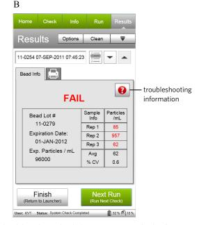
**Figures A and B.** Example Data: System Check bead data obtained with the Muse® System Check software module and acquired on the Muse Cell Analyzer. Figure A shows passing results, while Figure B shows results that failed. Results include the bead count for each replicate, average bead count, and %CV. Bead counts (Particles/mL) that fall outside  $\pm 10\%$  of the expected value appear in red.
