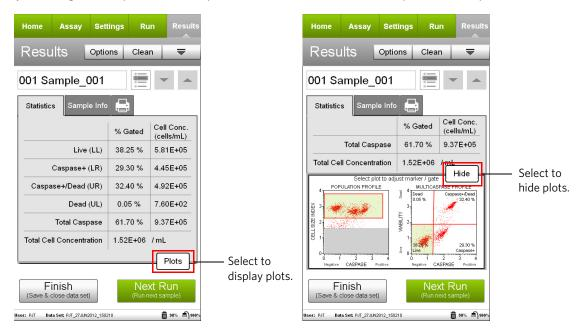
12. (Optional) If changes are needed to the gate or markers, touch a plot to enlarge it, then adjust the cell size gate or markers, as described in steps 4 and 6, respectively. You cannot adjust the cell size threshold after the sample has been acquired.
