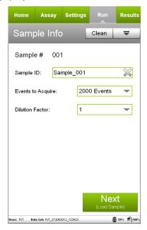
10. Mix the first sample and load it on the instrument. Select **Run** to run the sample.
