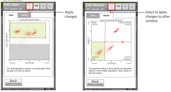
13. If no adjustments are needed, select **Next Run** and repeat steps 9 through 12 for the remaining samples.
