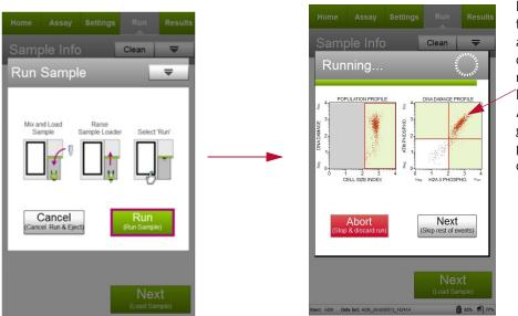
During acquisition, live statistical values are generated and represented on a dot plot graph. Quantitative measurements include Negative, single positive ATM phosphorylation, single positive H2A.X phosphorylation, and DNA double-stranded breaks 11. When acquisition is complete, the results are displayed. If desired, select **Plots** to display a dot plot and a bar graph for the sample.
