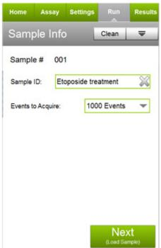
Follow the onscreen instructions and mix the first sample. Load the sample on the instrument loading arm. Select **Run** to acquire the sample.
